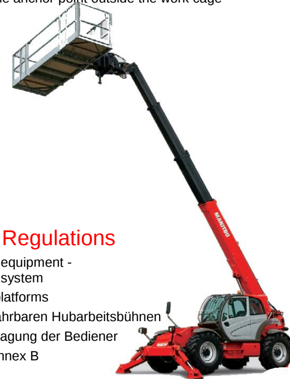
4 Multifunctional device with pivoting work cage and suitable inward opening access gate.
