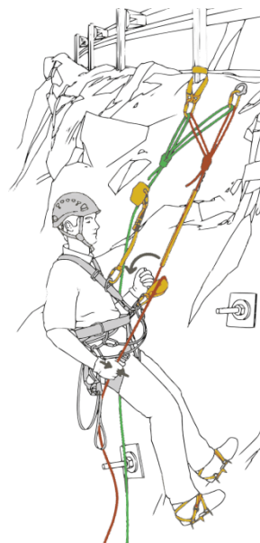
2: Redundancy means: Using two independent ropes simultaneously, which have separate anchor points. (Illustration: Petzl)
